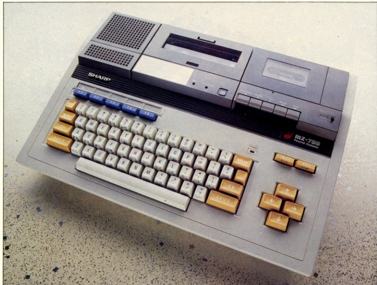
The front of the Sharp MZ 731 (above) shows the keyboard layout and the integrated speaker, plotter and cassette deck from left to right across the top. The close-up of the cassette deck (right) shows how compact it is, despite its taking standard audio cassettes. Below it can be seen the insert and delete keys and the power light.
